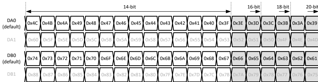
Figure 8-44. 1-wire output bit mapping
